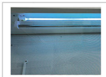
UV Lamp Emission of 253.7 nanometers for most efficient decontamination. The radiation intensity is not less than 400mW/m 2 .
